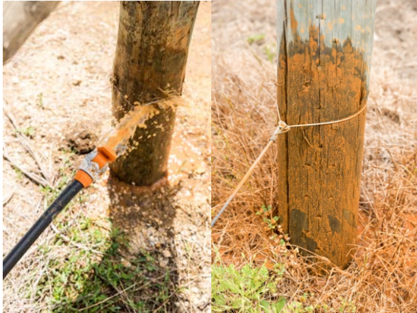
Iron precipitate ejected from a dripper line during flushing in the Limestone Coast. Photos: Gavin Blacker.
