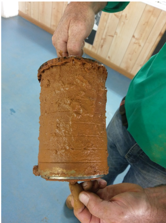
A pump component from the Limestone Coast region affected by an iron precipitate. Photo: Lawrences Irrigation.
