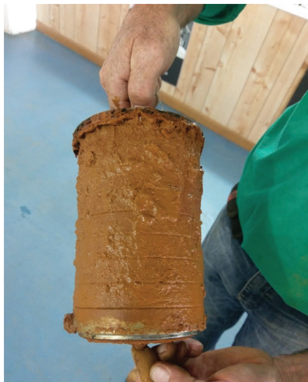
A pump component from the Limestone Coast region affected by an iron precipitate. Photo: Lawrence's Irrigation.
