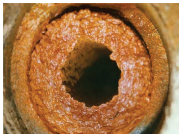
100 mm pipe clogged with an iron bacteria biofilm. Source: SA MDB NRM Board (2006).
