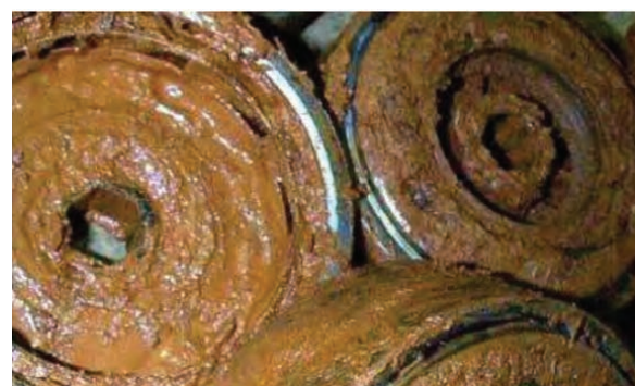
Iron biofouling of a submersible pump. Source: Forward (2008) in GHD (2010).
